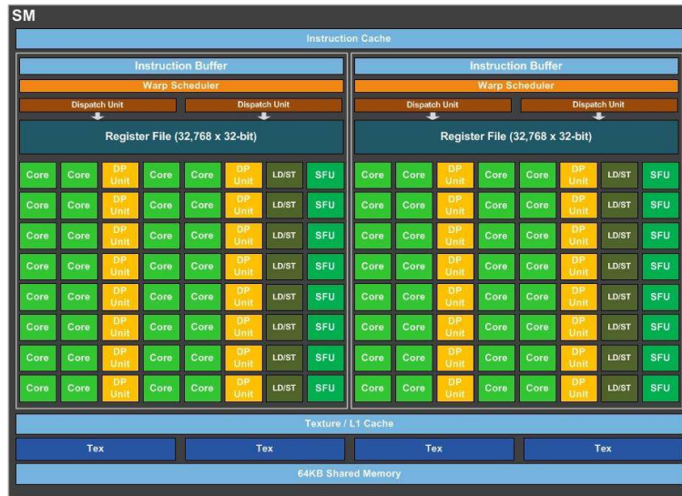
FIGURE 2.2: Architecture of a single NVIDIA GP100 SM (Source: NVIDIA Tesla P100 Whitepaper [35])
