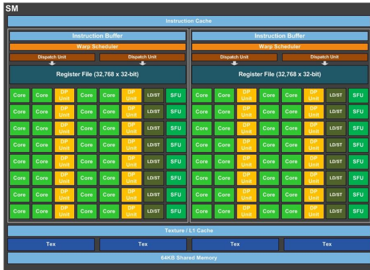
FIGURE 2.2: Architecture of a single NVIDIA GP100 SM (Source: NVIDIA Tesla P100 Whitepaper [40])
